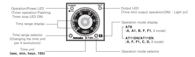
\*Please rotate the time range switch and operation mode switch to CW(Clockwise) direction.
