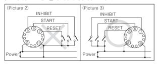
3) When using more than one timer with one contact or transistor input. Please connect the power phase correctly.
