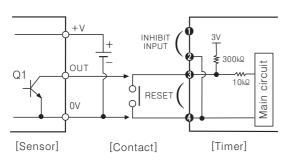
**※②**, **④** are GND terminals and connected inside.
