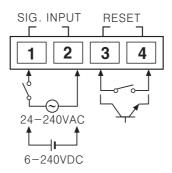
\*\*Power terminal (No. 1, 2) and Reset terminal (No. 3, 4) are isolated.
