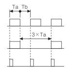
Therefore Ta(ON width) and Tb (OFF width) need to be over min. signal width.
